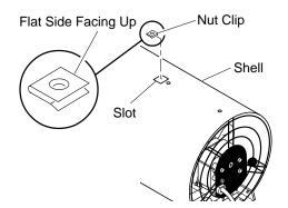
Figure 4 - Installing Nut Clip
